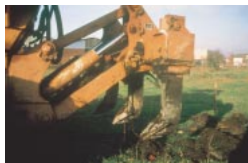
Tractor-mounted wing tines rip through compacted ground and improve drainage
