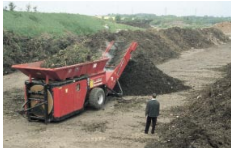
The material is shredded and left in windrows to compost - £1 million worth of capital investment in specialist machinery and hardstanding
