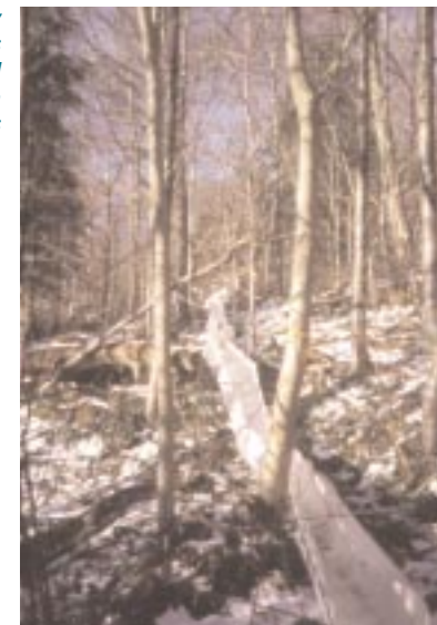
Heavy duty polythene log chutes cause minimal damage, even on steep slopes
